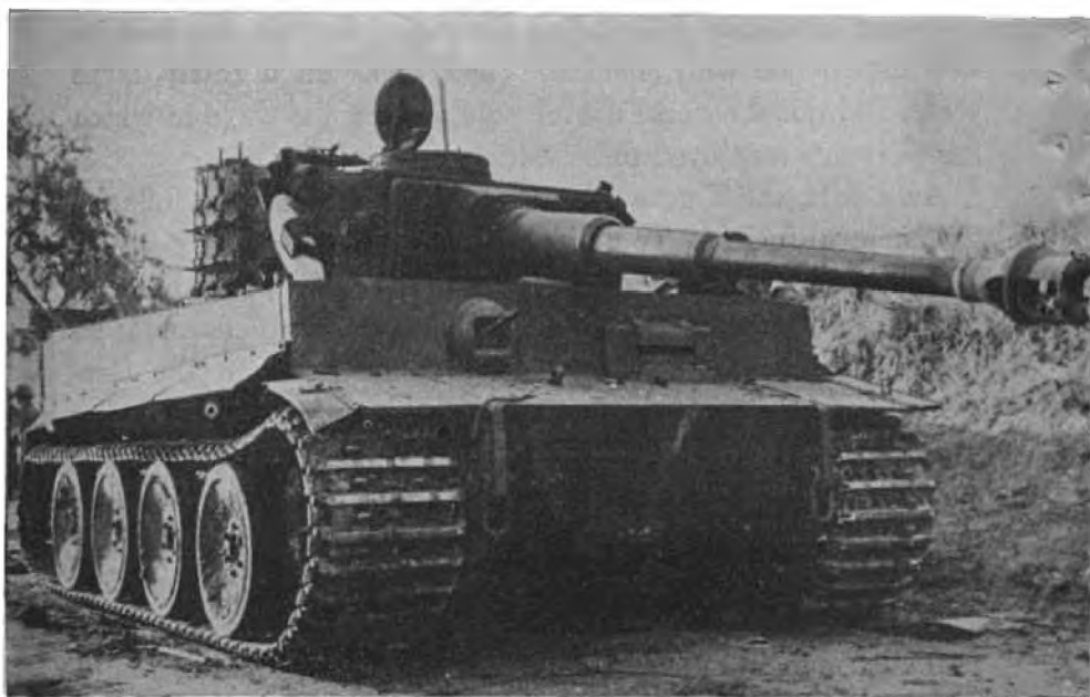
This is a standard Tiger tank — or, as the Germans designate it, Pz. Kpfw. Tiger. (The Roman numeral "VI" has been dropped.)
