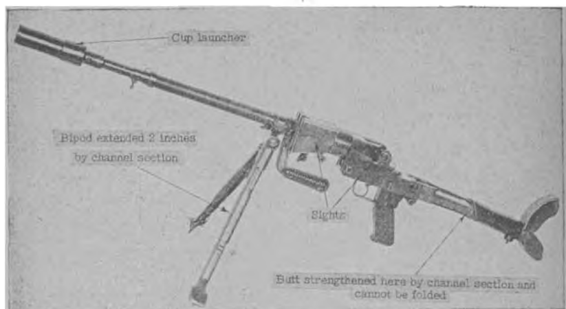
The antitank rifle modified into a grenade discharger.
