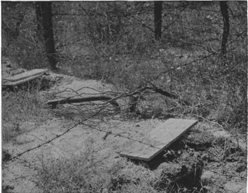
A fougasse flame thrower emplaced under a barbed-wire entanglement. Only the nozzle and propellant cylinder show above ground.
