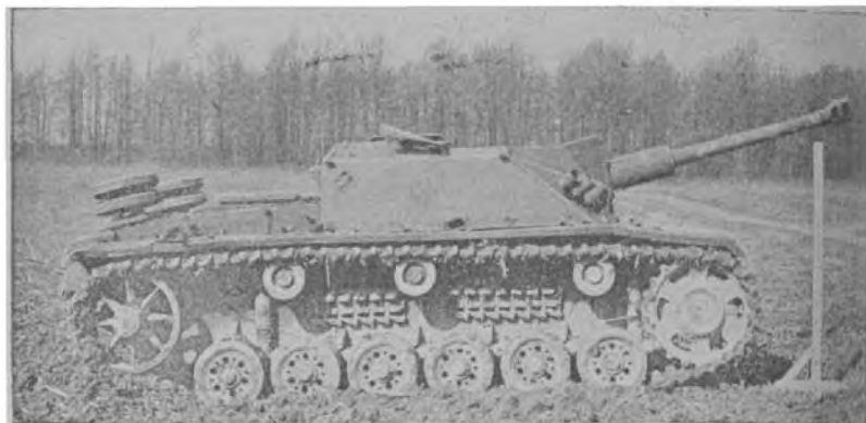
A side view of the widely used 75-mm assault gun, 7.5-cm Stu. G. 40 .
