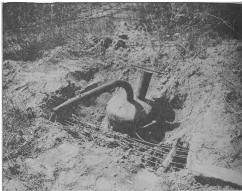
A fougasse flame-thrower emplacement, partly uncovered, showing the control wires leading to a central switchboard.
