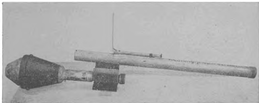
The Panzerfaust 30 , with sight raise and projectile shown separately. The projectile vanes are extended.
