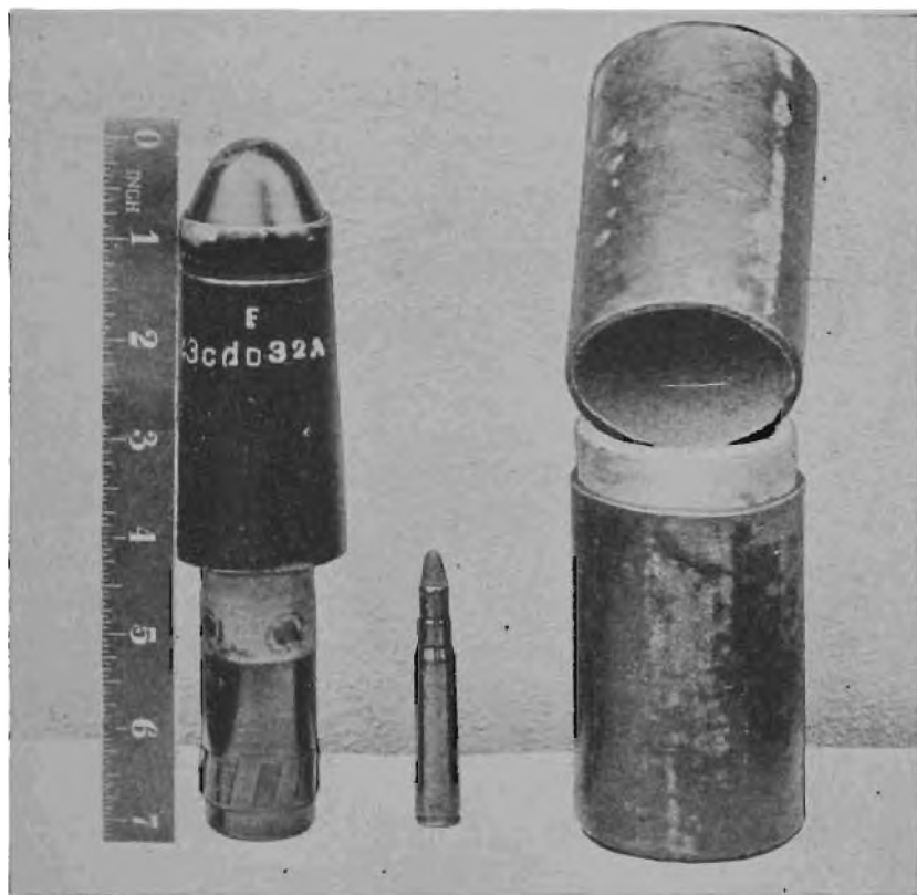
Figure 11. Large Hollow-charge Antitank Grenade, Propelling Cartridge, and Carton.
