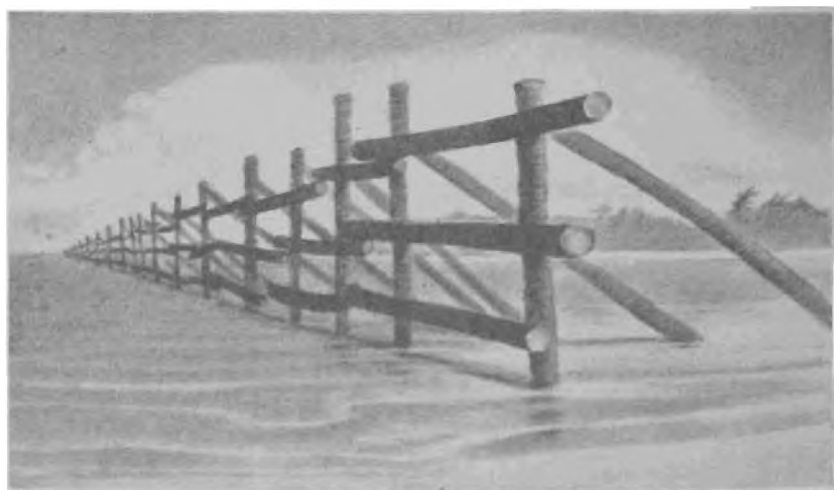
Figure 2.—Japanese Antiboat Barricade.
