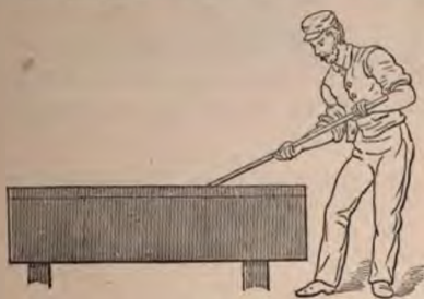
FIG. 15.—WASHING THE GUN-COTTON.
