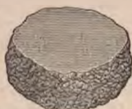
FIG. 41.—CAST LEAD PLUG AFTER COMPRESSION.
