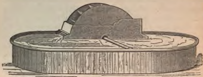
FIG. 18.—POACHER FOR WASHING GUN-COTTON PULP.
