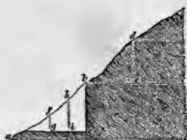
FIG. 69.—BLASTING ON AN INCLINE.
