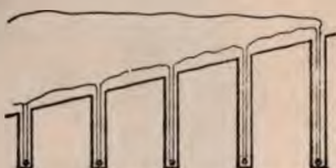
FIG. 91.—MINES ELECTRICALLY CONNECTED.
