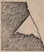
FIG. 66. — BORE-HOLE NOT BOTTOMED.
