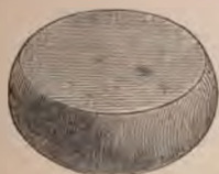
FIG. 40.—DRAWN LEAD PLUG AFTER COMPRESSION.
