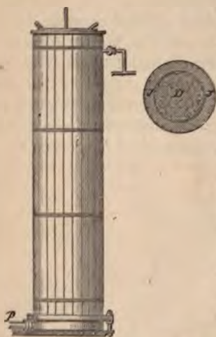
FIG. 13.—DRYING CYLINDER AND SECTION OF DRYING TUBE.
