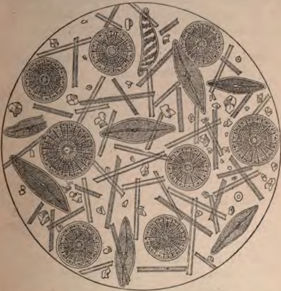
FIG. 7.—KIESELGUHR DYNAMITE UNDER THE MICROSCOPE: SAMPLE OF 1872.
