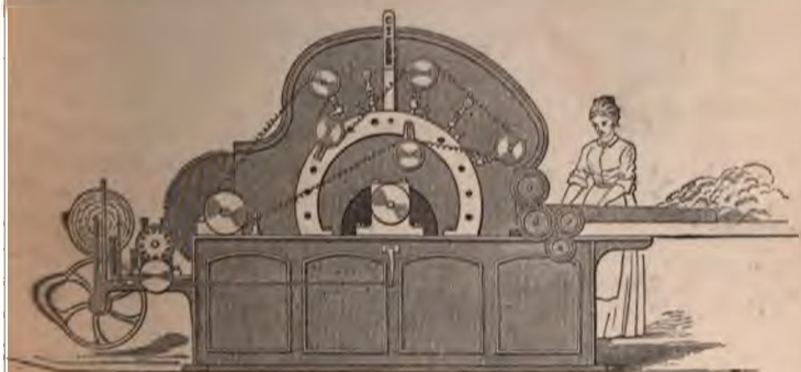
FIG. 12.—CARDING MACHINE FOR GUN-COTTON.
