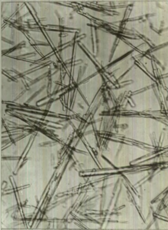
FIG. 11. R.N.C.F. NORMAL SPRAYED PICRITE S_o = 21,000 \text{ cm.}^3/\text{cm.}^3
