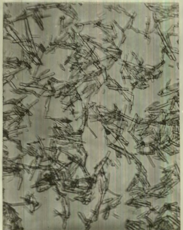
FIG. 12. R.N.C.F. PRESSURE SPRAYED PICRITE S_o = 38,000 \text{ cm.}^3/\text{cm.}^3
