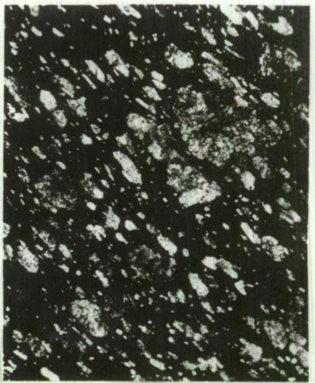
FIG. 9. F527/30 CORDITE N. CARBAMITE DISSOLVED IN THE SOLVENT
