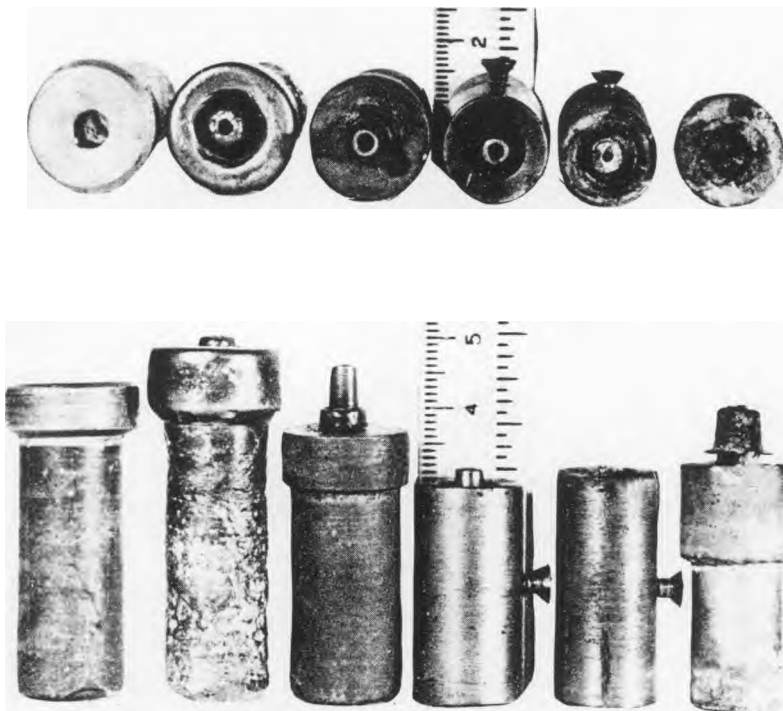
Figure 175. Assorted Fuze Striker Assemblies.
