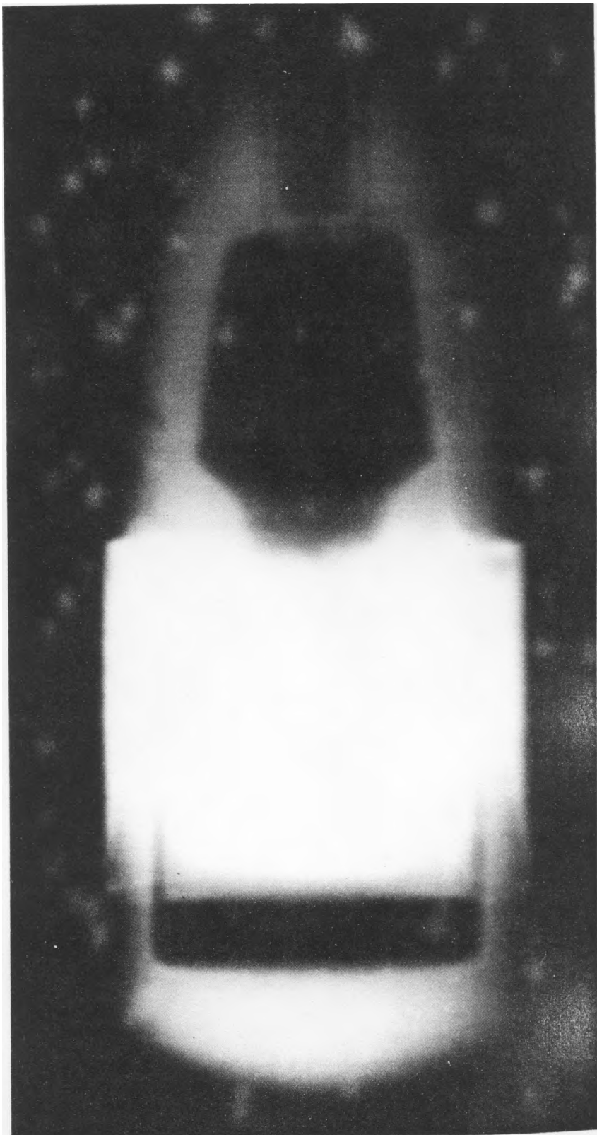
Figure 73. Radiograph of 4-Inch Hotchkiss Shell.
