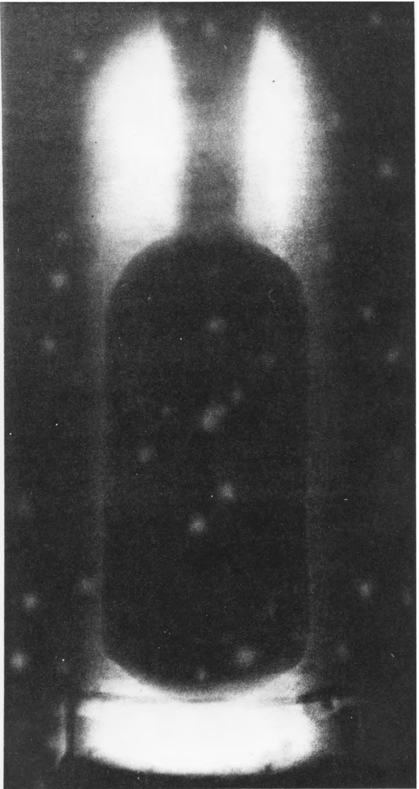
Figure 50. Radiograph of 3-Inch Read-Parrott Shell (Figure 48).
