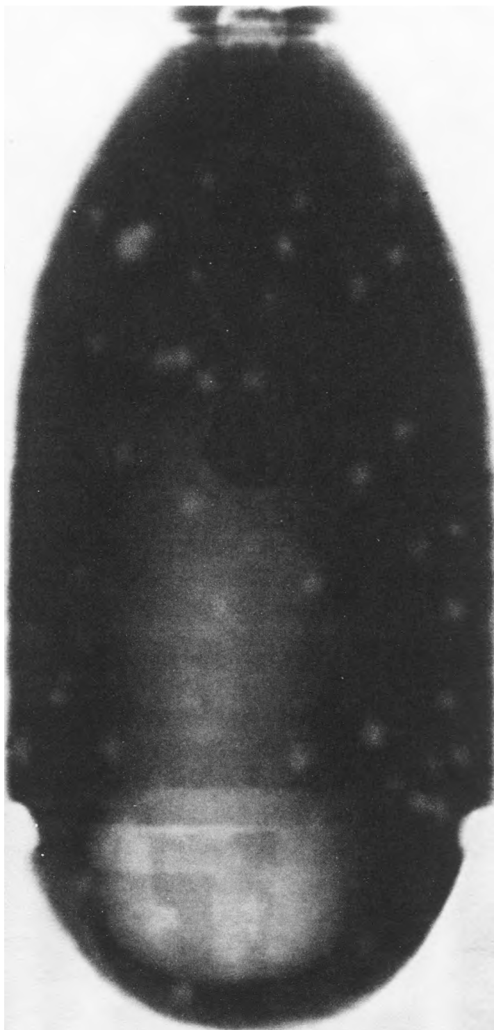
Figure 37. Radiograph of 4.2-Inch Dahlgren Shell (explosive).
