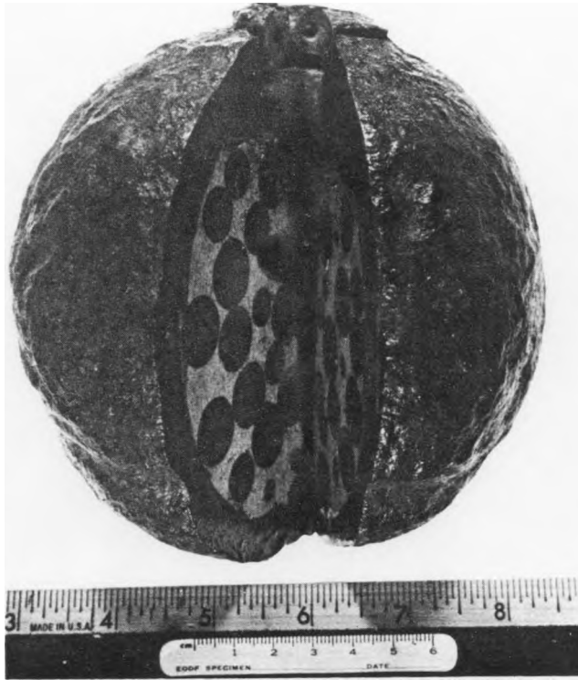
Figure 9. 24 Pdr. Case Shot, Sectionalized.
