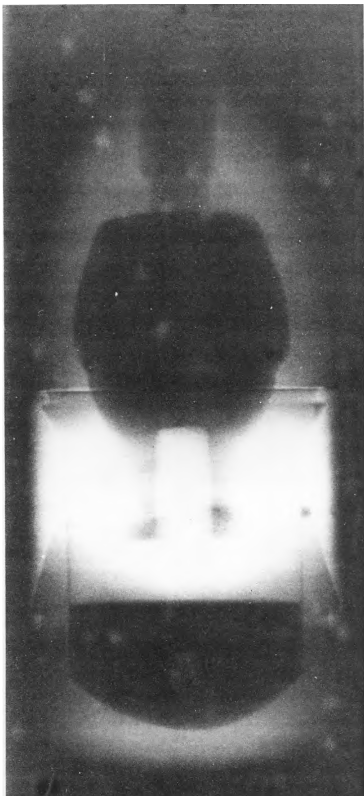
Figure 65. Radiograph of 3.4-Inch Hotchkiss Shell.
