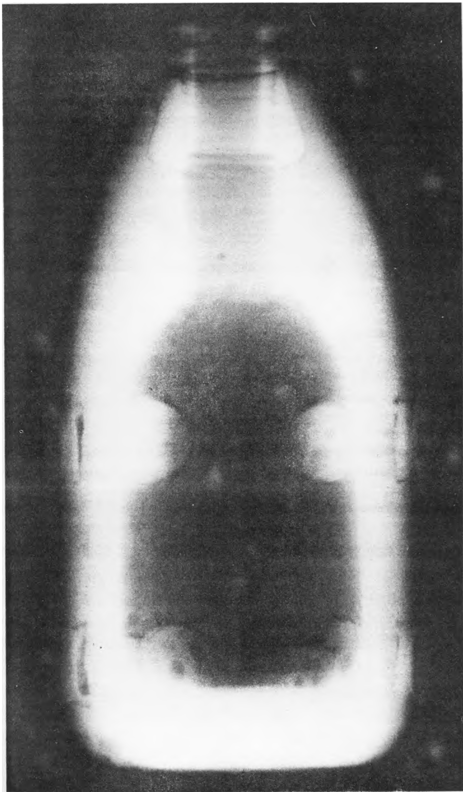
Figure 21. Radiograph of 3.5-Inch Studded Blakely Shell.
