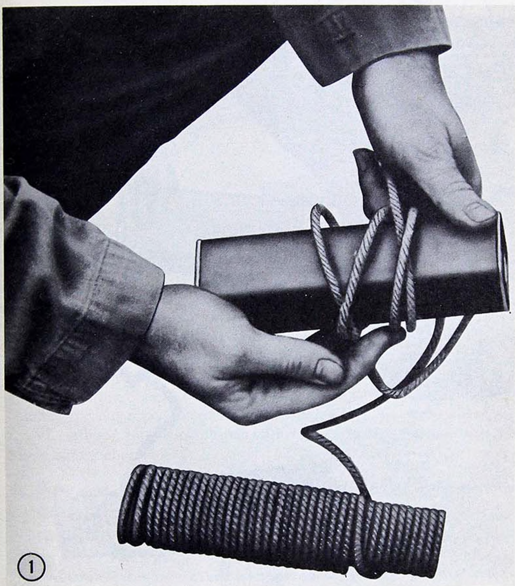
Figure 57. Priming TNT block and dynamite with detonating cord.
