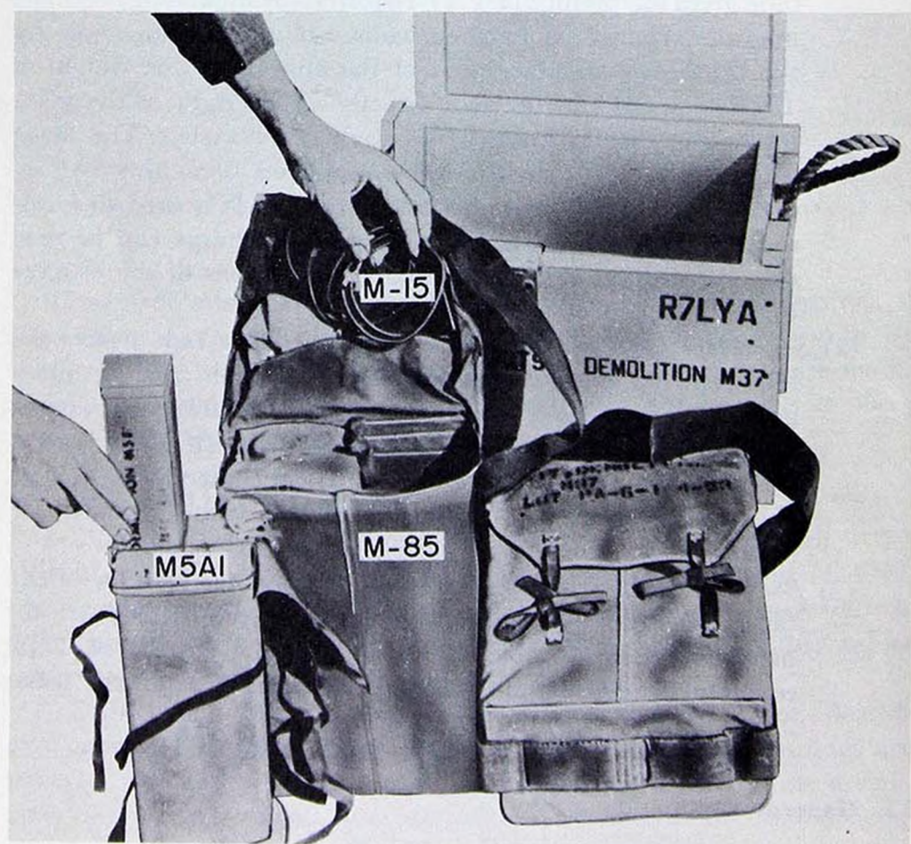
Figure 37. M-37 demolition kit.
