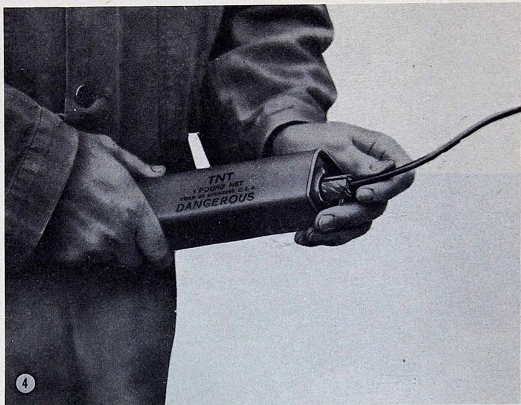
4 Inserting in threaded cap well. B—With nonelectric cap—Continued.
