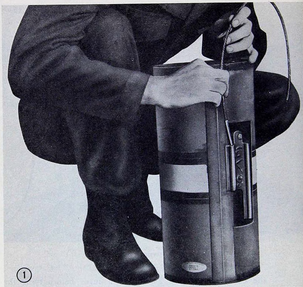
1 Inserting cap into well
