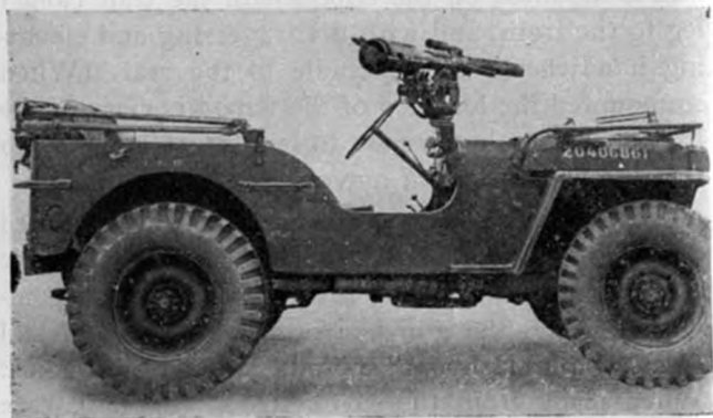
Figure 29. 57-rifle on dash mount, 1/4-ton truck.
