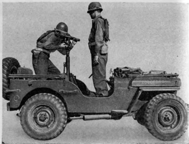
Figure 28. 57-mm rifle on pedestal mount, 1/4-ton truck.
