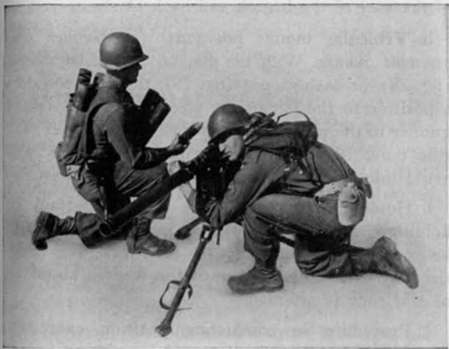
Figure 48. Positions of gunner and assistant gunner, 57-mm rifle mounted on machine gun tripod M1917A1.
