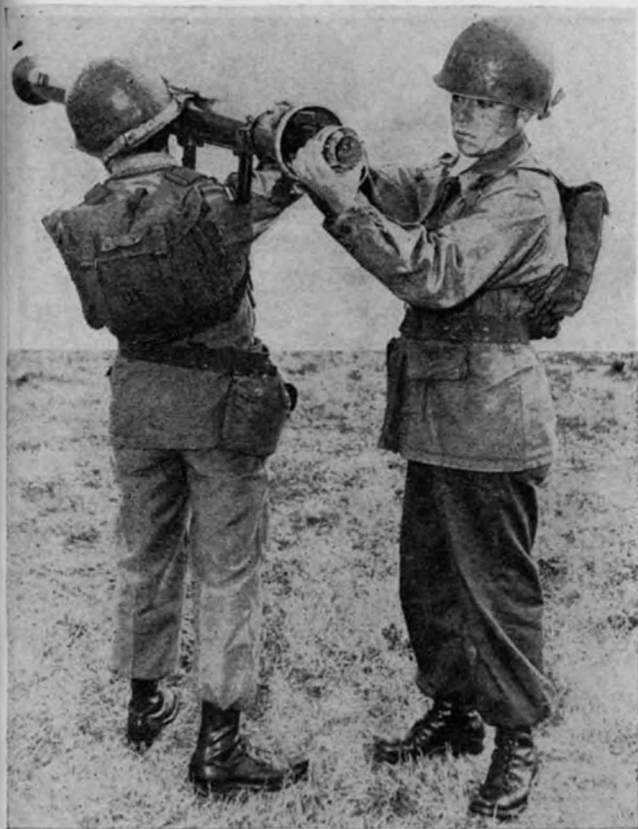
Figure 54. Slide rocket into launcher and press the contactor latch.
