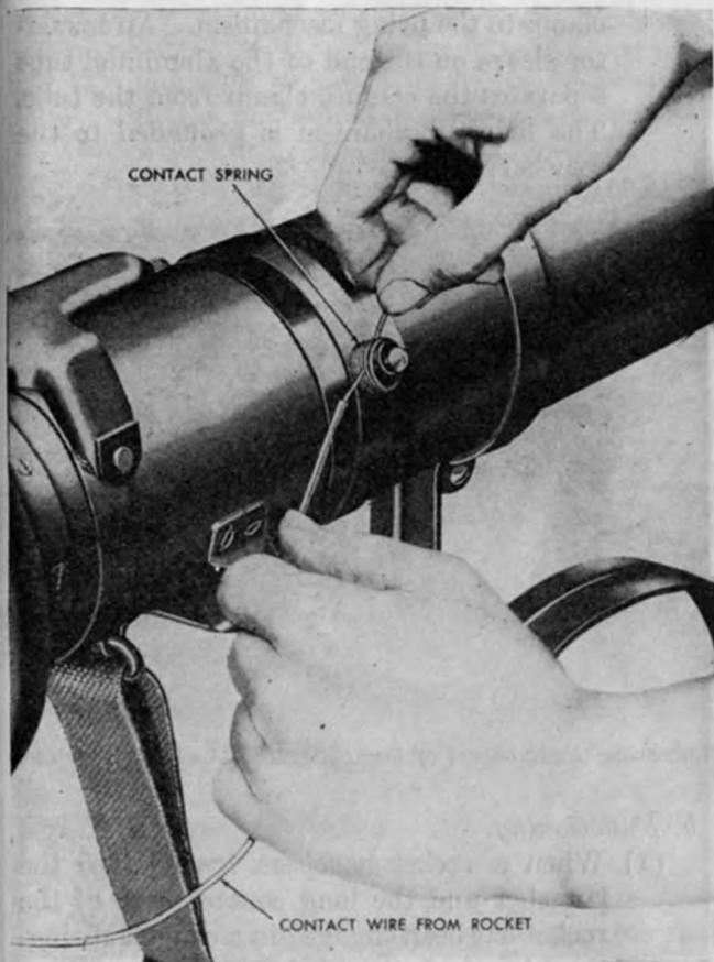
Figure 51. Placing contact wire to contact spring.
