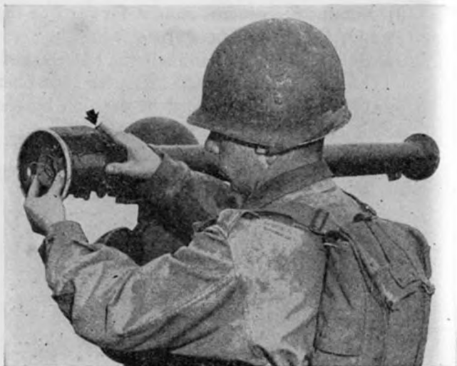
Figure 39. Control handle in LOAD position with rocket inserted.
