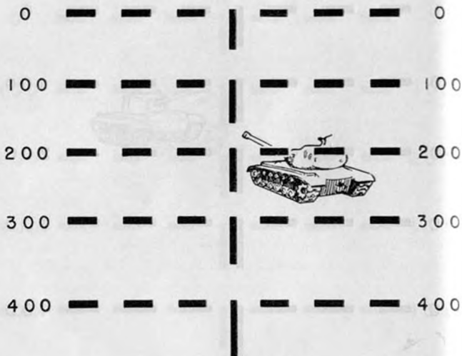
Figure 31. Target, 200 yards away, moving away from the gunner from the right front toward the left at an angle of 60° and at 20 m. p. h.
