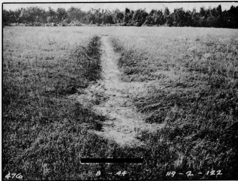
FIG. 10. Cleared path after 13 strands of detonating cord has been detonated in Schu mine field.
