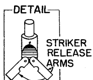
TYPE 90 FLARE IGNITER MODIFIED FOR USE IN AERIAL BOMB
