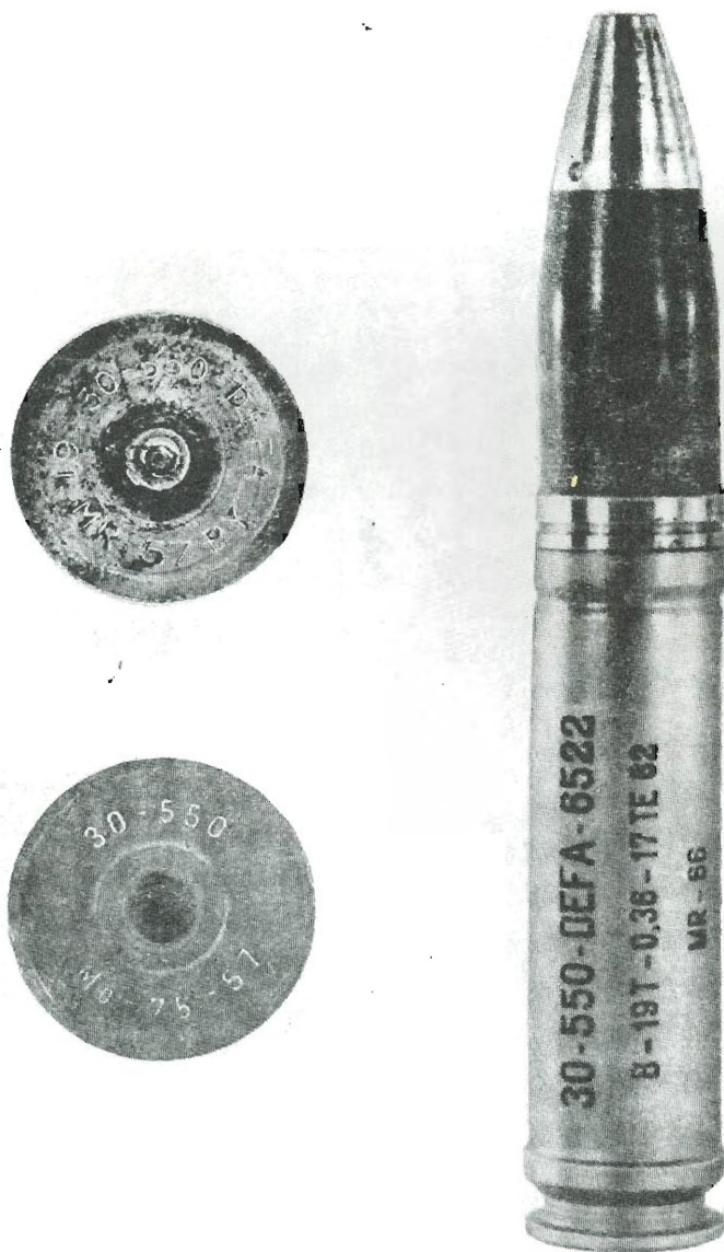
Figure 9. French cartridge markings.
