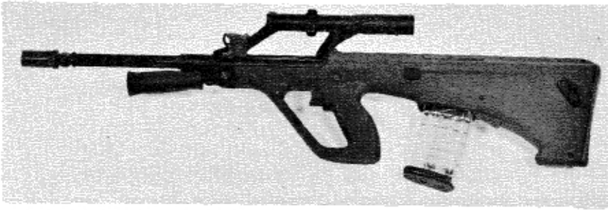
Figure 103.1. Austrian 5.56-mm St.G 77 (AUG) assault rifle with 508-mm barrel.
