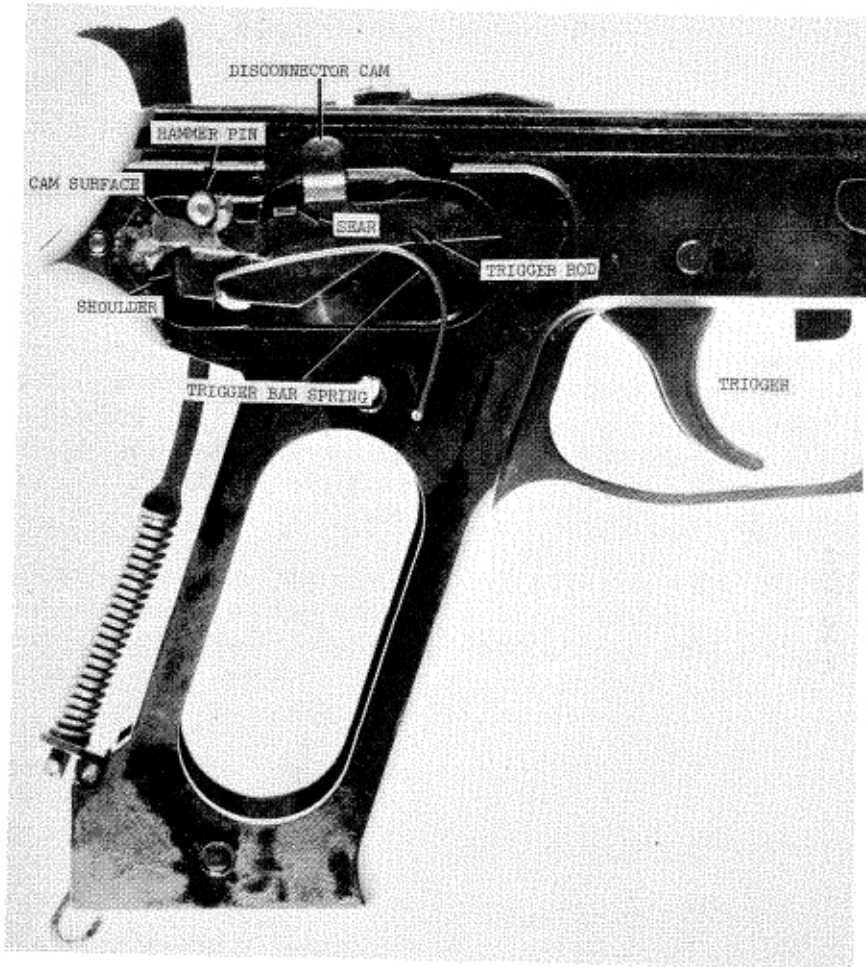
Figure 28.1.5. Model 75 trigger mechanism, at rest.
