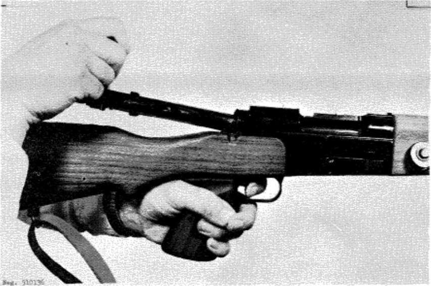
Figure 137. FR-F1 bolt removal.
