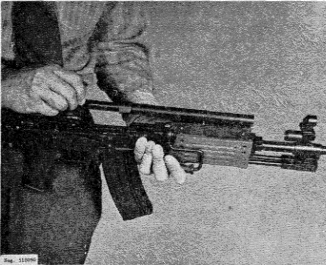
Figure 91. Removing gas cylinder tube.
