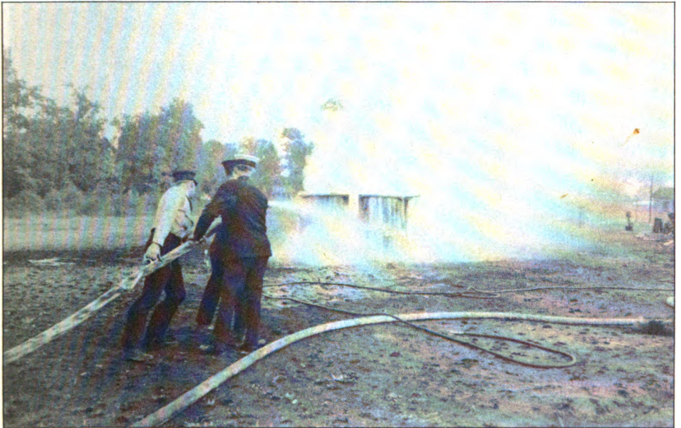
Same fire as previous picture. Water started at 64 sec. after ignition resulted in a minor explosion causing roof to fall in. Picture at 94 sec. Fire out at 120 sec.
