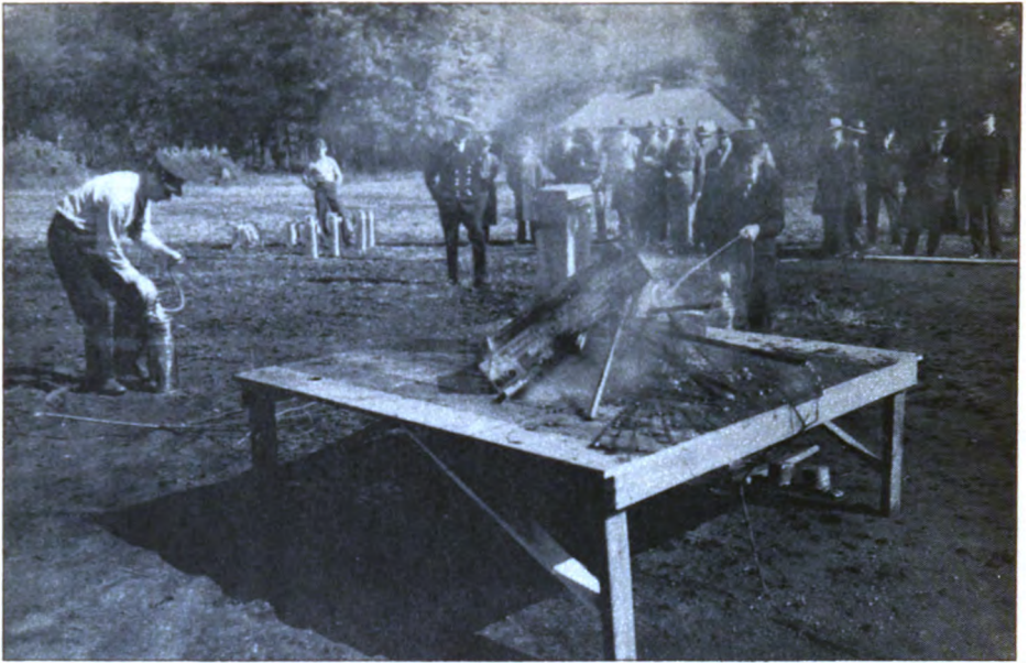
A fire was produced in a pile of kindling and shell boxes by an 8-lb. thermite incendiary bomb. This picture was taken after three 2½-gal. extinguishers had been used.
