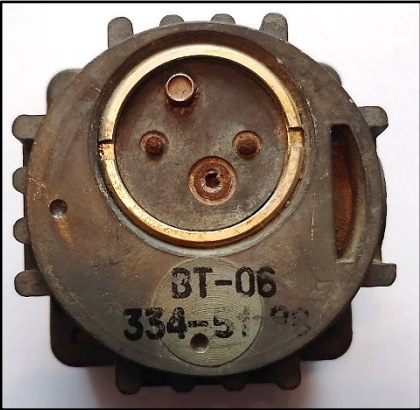
VT-06 (magnetic-influence) Height of body: 76mm Width of Body; 76mm
