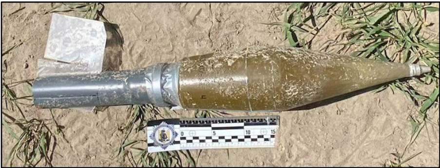
KZ-6 Shaped Charge Adopted as Drone-dropped Munition (HEAT)
