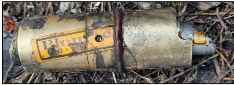
Electromechanical fuze for Shahed-136 / Geran-2 UAV (impact)
