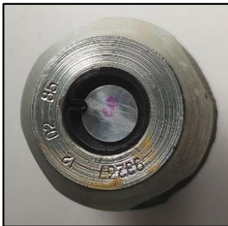
9E237 (impact, pyrotechnic delay) Diameter: 49.95mm Length without detonator: 58.3mm Country of origin: USSR
