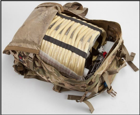
MPLC (mine-clearing system) Country of origin: USA
