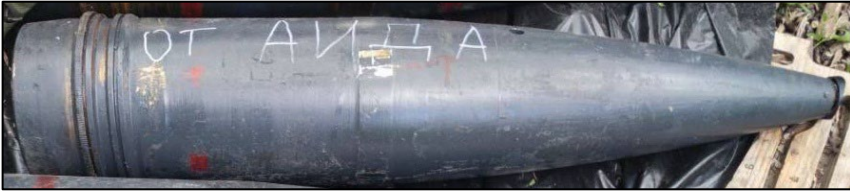
170mm North Korean projectile (model unknown) (HE-frag)
