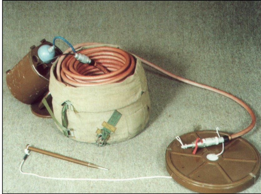
ZRP-2 "Trail" (mine-clearing system) Country of origin: russia
