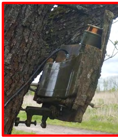
MVE-92 Diameter: 86mm Length: 50mm Country of Origin: USSR
