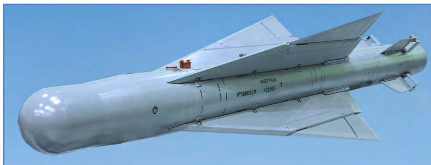
UPAB-1500B-E / K029BE Diameter: 400mm Length: ~ 5m Weight: 1525 kg Country of Origin: Russia
