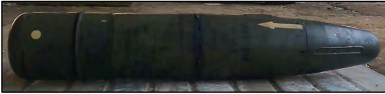
9M119M "Reflex-M" Unfired Diameter: 125mm Fired Length: 760mm Country of Origin: Russia
