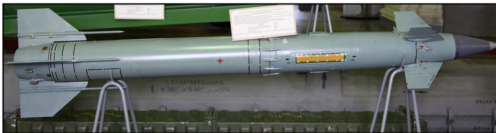
9M330 "Tor" Diameter of Body: 235mm Length: 2898mm Wingspan: 650mm Country of Origin: Russia
