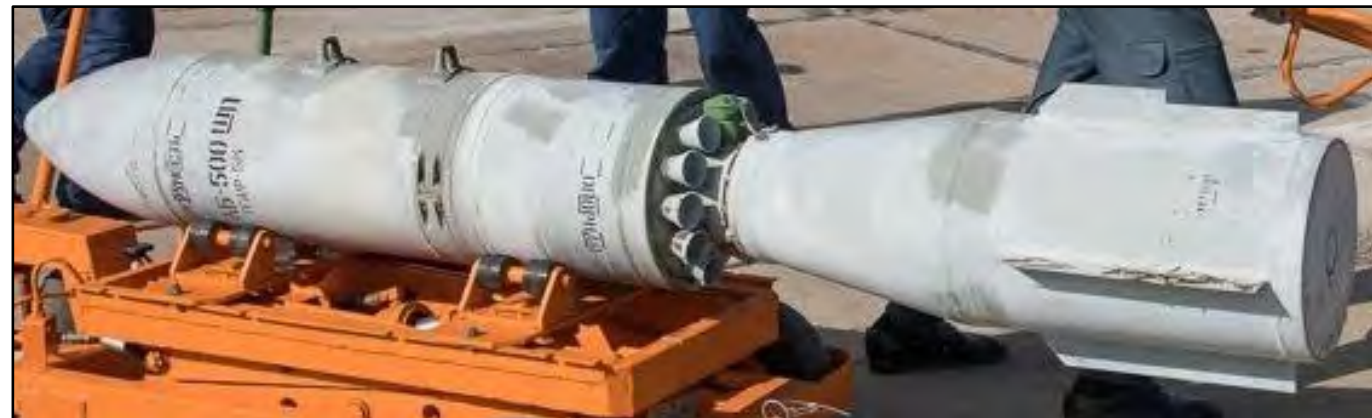
BETAB-500ShP Diameter: 325mm Length with Parachute Assembly: 2510mm Weight: 380 kg Country of Origin: Russia
