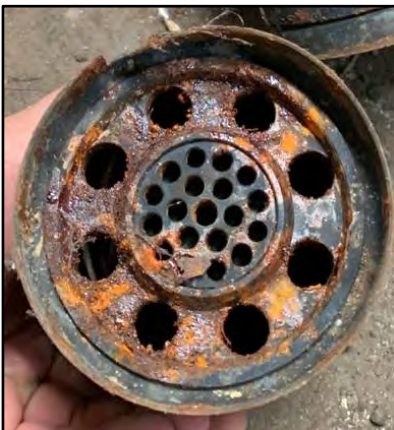
Launch Motor for RPO-A Diameter: 90mm Length: 210mm Country of Origin: Russia
