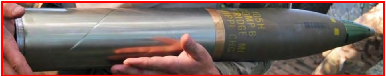
105mm M1 (HE-Frag) Length of Projectile: 400mm Length with Cartridge: 725mm Note: Uses the M739A1 Fuze. Country of Origin: USA
