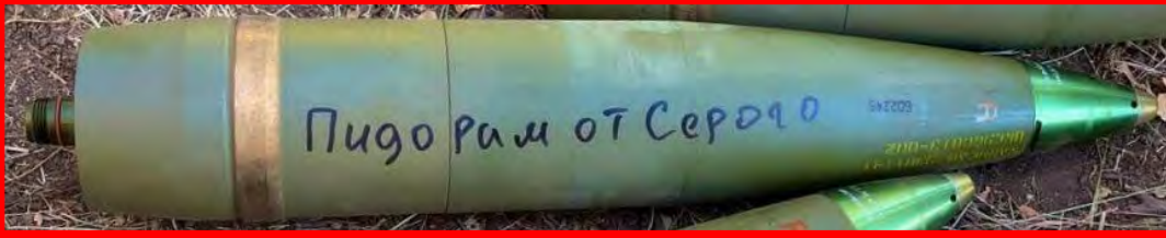
105mm M927 (Rocket-assisted HE-Frag) Length without Fuze: 539mm Note: Uses the M739A1 Fuze. Country of Origin: USA
