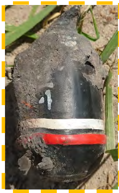
Combined Effect Cluster Hand Grenade RGK-60KD Diameter: 58mm Length: 173mm Country of Origin: Russia
