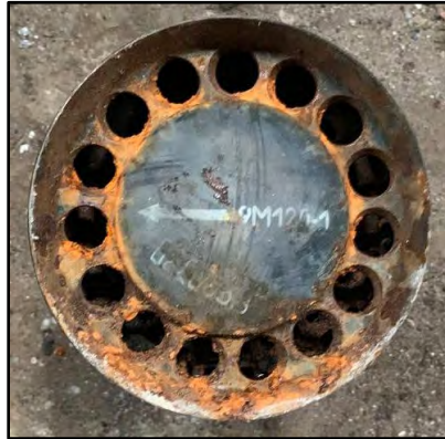
Launch Motor for RPO-A Diameter: 90mm Length: 210mm Country of Origin: Russia
