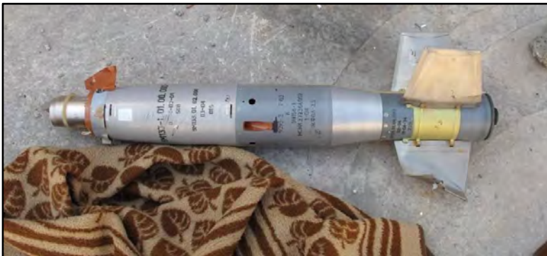
9M119M "Reflex-M" Unfired Diameter: 125mm Fired Length: 760mm Country of Origin: Russia
