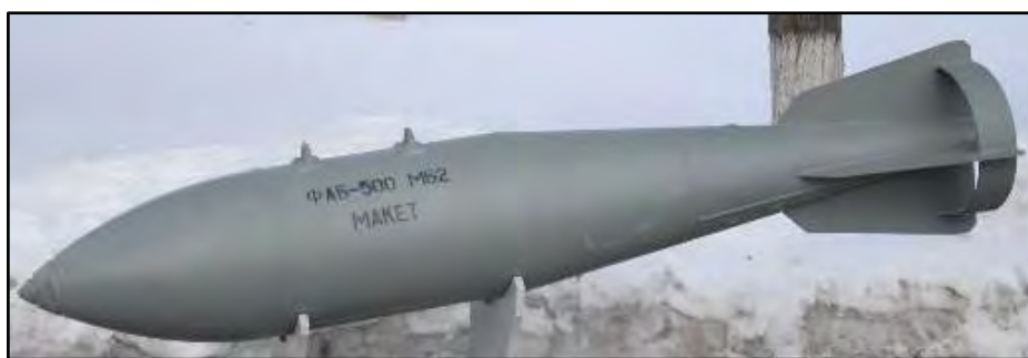
FAB-500 M-62 Diameter: 400mm Length: 2470mm Weight: 497 kg Country of Origin: Russia
