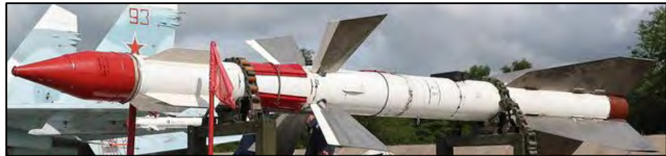
Warhead of the K-13/R-13 Missile (NATO AA-2) Diameter: 127mm Length: 765mm Country of Origin: USSR
