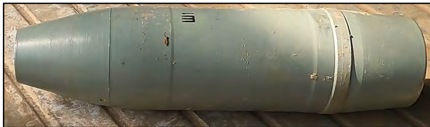
122mm Sh-1 (Flechette) Length of Projectile: 455mm Country of Origin: USSR
