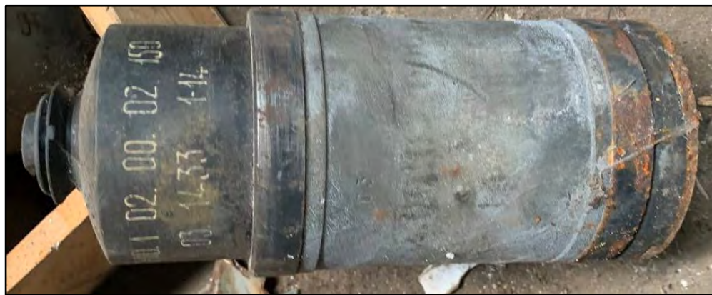
Launch Motor for RPO-A Diameter: 90mm Length: 210mm Country of Origin: Russia
