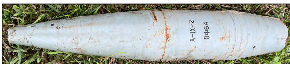
152mm OF64 (HE-Frag) Length without Fuze: 802mm Length with V-429 Fuze: 860mm Country of Origin: Russia
