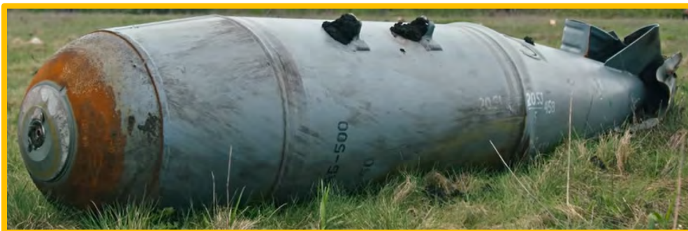
OFZAB-500 Diameter: 450mm Length: 2385mm Weight: 500 kg Country of Origin: Russia
