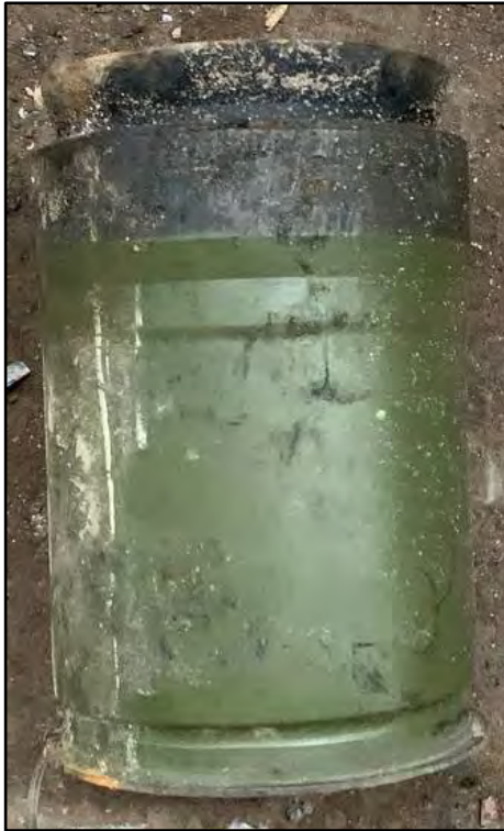
Launch Motor for RPO-A Diameter: 90mm Length: 210mm Country of Origin: Russia
