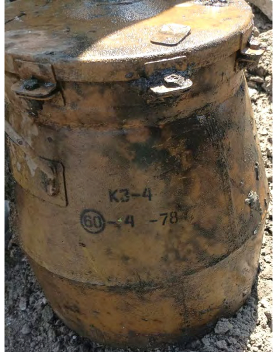
KZ-4 Diameter: 410mm Height: 440mm Country of Origin: Russia
