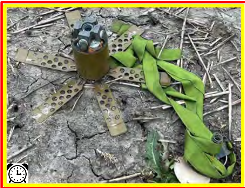
POM-2 Diameter: 63MM Height: 180MM Country of Origin: USSR/Russia
