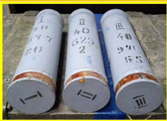
ZAB-2.5 Diameter: 68mm Length: 244-249mm
