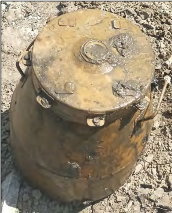
KZ-4 Diameter: 410mm Height: 440mm Country of Origin: Russia
