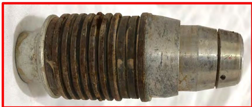
40mm VOG-25P (Bounding Fragmentation, Projected Grenade)
