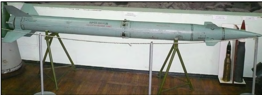
9M33 "OSA" Diameter: 206mm Length: 3158mm Country of Origin: USSR
