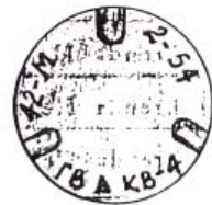
Figure 30. Allocation of and key to designators stamped into the metal body of fuzes and primers
