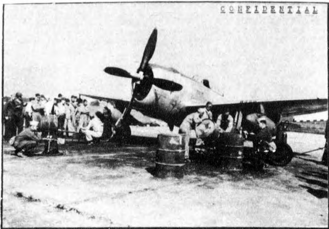
FIG. 12 FILLING TWO FIRE BOMBS, MOUNTED ON A P-47, WITH THICKENED FUEL USING FUEL MIXING AND TRANSFER KIT, E2.
