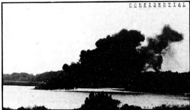
FIG. 15 FIRE BOMB, EQUIPPED WITH SODIUM IGNITER, FUNCTIONING ON WATER. SODIUM PARTICLES HAVE SURFACED AND BROKEN INTO FLAME SETTING FUEL AFIRE. (THIS PICTURE TAKEN AFTER SHEET OF FLAME HAD DIMINISHED.)
