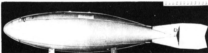
FIG. 5 F4U-1D, P38, PV WING PYLON FUEL TANK WITH STABILIZER AND HARNESS. (NOTE, CLAMP FOR IGNITER)
