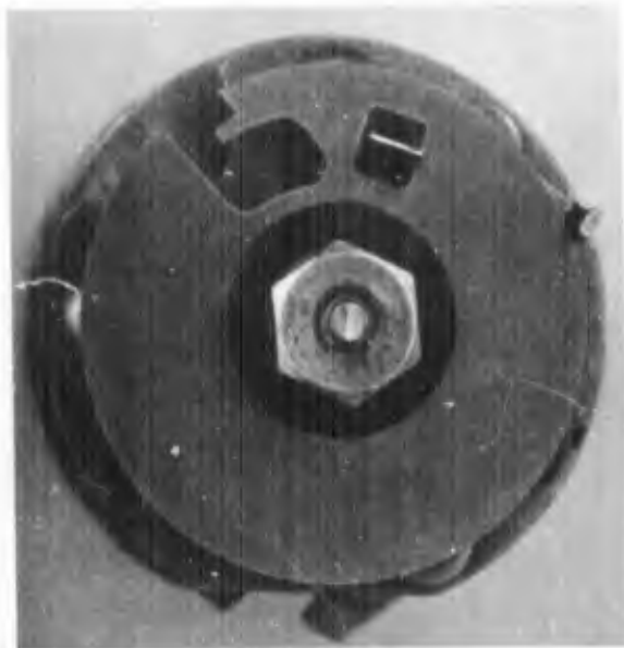
Figure 13. FMU-54A/B Fuze Timer Assembly - Top View
