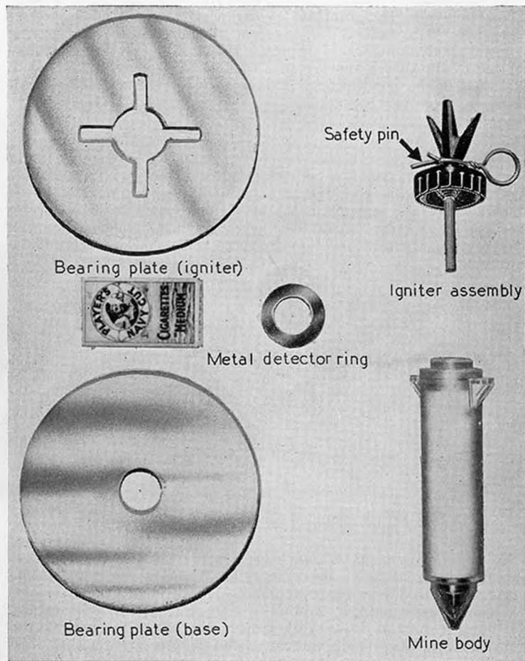
Fig 21.—Anti-personnel mine, No. 6—standard and special parts
