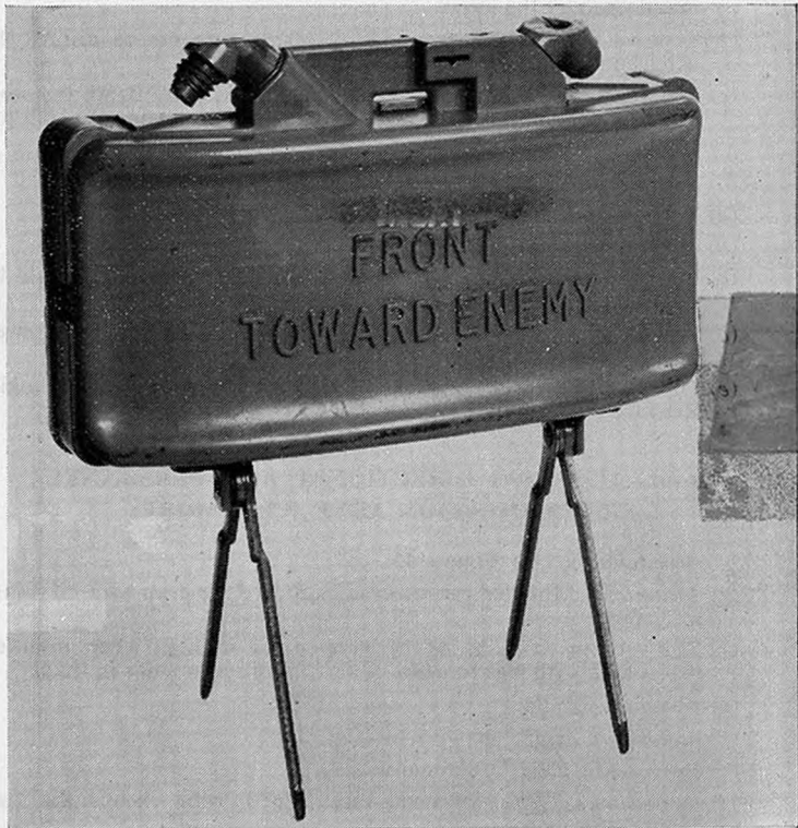
Fig 45.—M18A1 directional anti-personnel fragmentation mine
